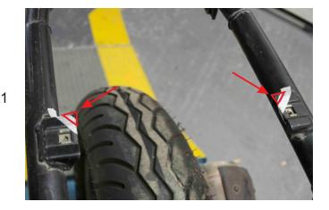
Remove the two triangular parts as shown in photo No1. Do not remove all the metal base sheet as you will need it to screw on the plastic cover.
