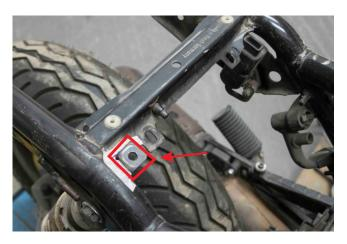
Remove also the square metal base as shown in photo No 2. You do not need to remove anything else in order to place the plastic cover. You will screw the plastic cover on the plastic clips located on the transverse metal base.
