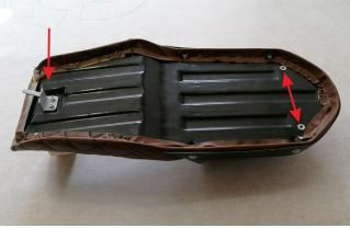
The seat cover has a small metal latch at the front
