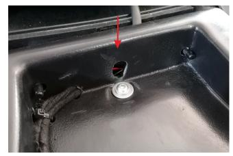
The hole on the plastic is used to support the seat cover at the front end
