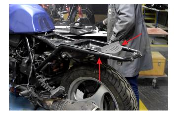
Place the metal plate (found in the installation pack) upside down on the plastic cover. Ensure that its holes are in alignment with the rear holes of the seat cover.
