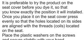
Place the plastic washers on the screws and secure slightly with your hand. Once you have placed all the screws secure them tightly.
