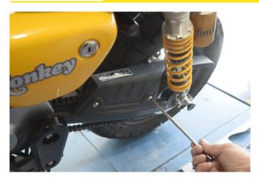
Remove the two screws holding the old chain guard and remove it from the motorcycle.
