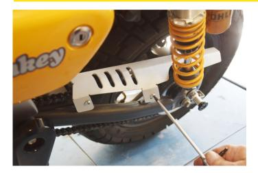
Place the new guard in the same position as old one. Screw it in with the new screws provided in the package.
