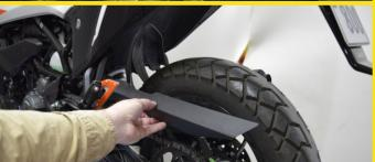
To place the new fender, you must remove the old one. In the photos you may find the order and the place of the screws you must remove.
