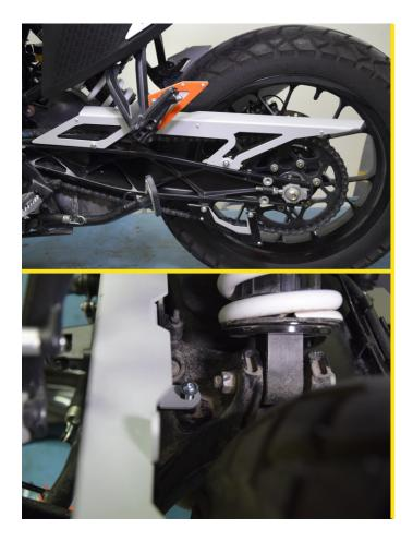
Put the chain guard in place and pass the screws (profile 4-8 front &3-5-6-7 for back) without tightening them, just touch them to hold the product in place.
