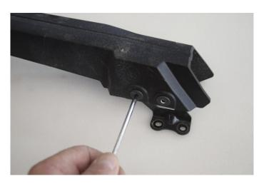
Remove the metal base that the protector has on the front part.
