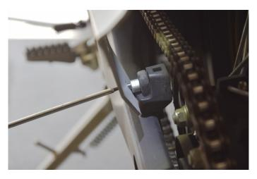
Slide the protector into place and screw it on back screw without tightening it.
