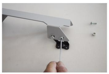
Screw it onto the new guard, but do not tighten the screws.
