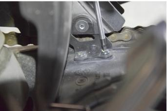
Unscrew the 2 screws holding the guard on the front and inside the scissor.
