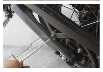
Then remove the screw that is visible from the outside, as shown on the photograph.
