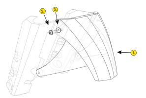
Basic condition for mounting this product you must first install the two fork guards (FG-KTM390). If these two are not present the product support is insufficient, and we do not recommend.
