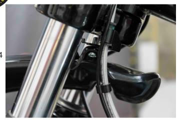
Put the fender in place and slide through the rear left screw. The cover support that holds the break tube, should be placed in between the fender and the triple clamp.
