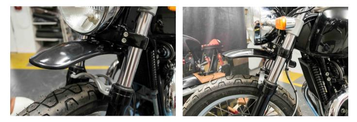
If you wish, you can remove the bridge from the old fender and use it with the newly placed fender. The end result should appear as in the photo Thank you for choosing one of our products.
