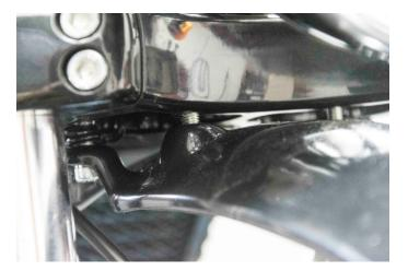
Place the front screws in the threads of the lower triple clamp and proceed to tighten all four screws tightly.
