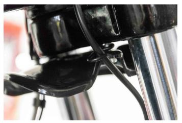
Repeat the same procedure on the right hand as well, placing once more the cover support of the break tube in between the fender and the triple clamp.
