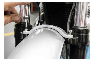
Undo the screws that the arrows in the left-hand photo show you and remove them. Keep the support covers that hold together the tubes- wires as we will use them later on.
