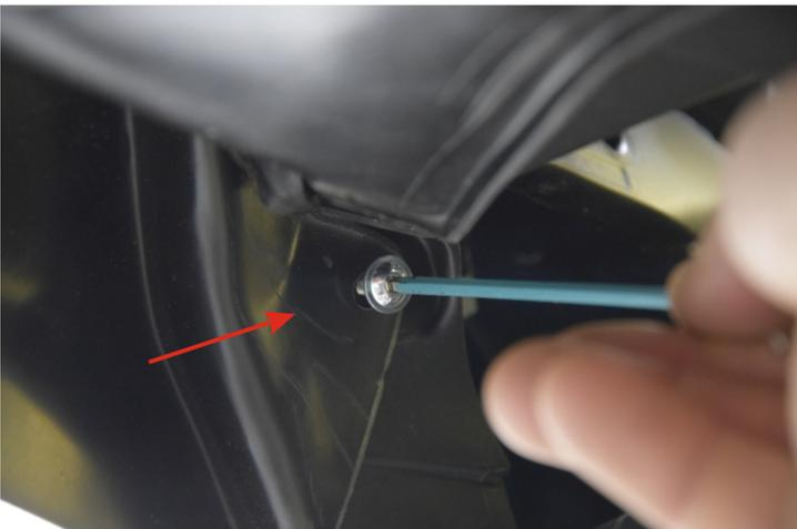
Remove the protective film on the back of the new fender and replace it. Screw the two small screws (M5X15) included in the package to the right and left of the fender on the inside as demonstrated in the photo. Just press the screws to hold the fender in place without tightening it properly.
