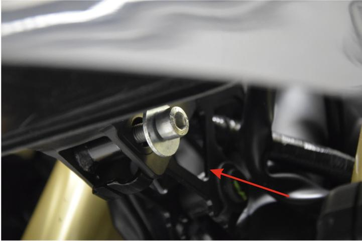
Remove only the bottom screw from the base that supports the lantern as shown in the photo. Store the screw and the clips, in case you want to restore the motorcycle to the original form.
