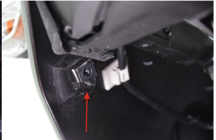
The inside of the fairing has a plastic part that extends to the bottom and is held by plastic clips (left photo). Remove the first upper clip and open the plastic to fit your hand. In the hole that fastens the clip, put the sliding thread that you will find in the package, mount it well and return the plastic to its position. Store the clip.
