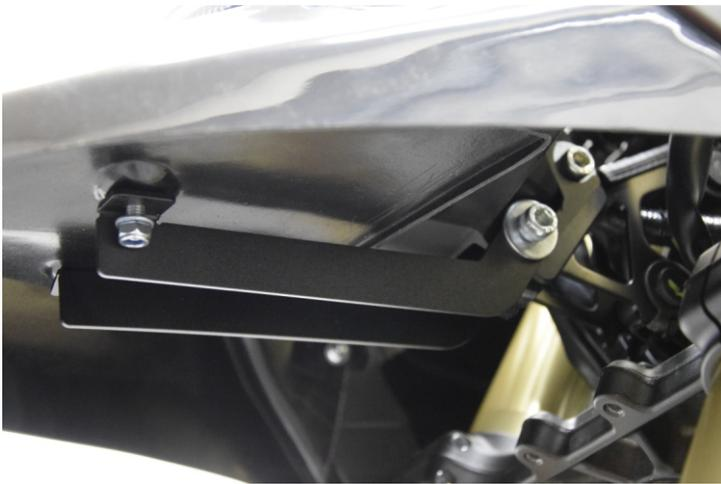
Install the two metal bases on the package exactly as shown in the photo. This is an extra support for the fender. Tighten the screws (M6X15) first and then the center screw on the base of the lantern. Finally, tighten the two side screws that secure the ferrules. Pay special attention to the central screw being tight.
