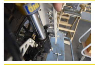
Do the same forthe top screw. Continue with the other side and after you have placed all the screws, check if they are aligned, then tighten them all.
