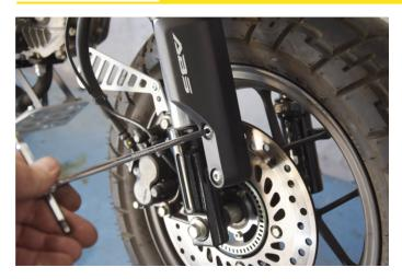
Remove the two screws holding the old protector and remove the it from the motorcycle.
