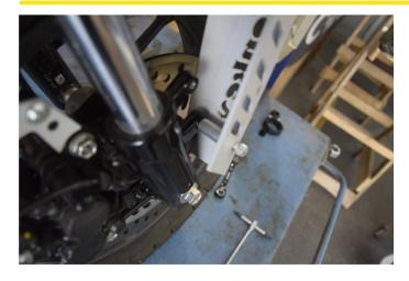
Place the adapter between the forks and the fork guard and screw without tightening.
