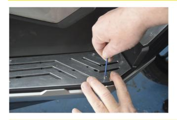
Place each part in its place, making sure it goes through the correct hole in the base. Screw in the screws while pressing the part down, as shown in the photo, so the nut does not turn on itself. Verify that you have tighten all the screws very well.
