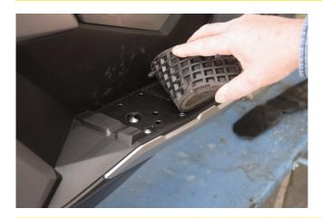
Remove the rubber cover of the footrest.
