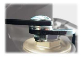
MOUNT THE WINDSHIELD/SCREEN ON THE BRACKET (PICTURE 1). REMOVE THE FIXING SCREWS OF STREERING PLATE, INSERT THE THICKNESS HIGH 13 INTO THE SCREW POSITION, APPROACH THE "B" STIRRUP AND INSERT THE 8X45 SCREW (PICTURE 2). DON'T LOCK. MOUNT THE WINDSHIELD/SCREEN WITH THE BRACKET MOUNTED BEFORE ON THE "B" STIRRUP USING THE "SQUADRE SHAPE" SCREW DIAM-ETER 6, THE WASHERS AND THE AUTOLOCK NUT (PICTURE 3).
