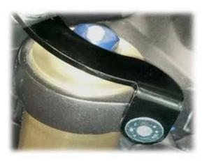
MOUNT THE WINDSHILED/SCREEN COMPLET-ED WITH BRACKET ON THE "b" STIRRUP MOUNTED BEFORE. USE THE LARGE WASHER AND THE AUTOLOCK NUT LIKE SHOWN IN THE PICTURE.
