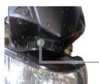
REMOVE THE CENTRAL FIXING SCREW OF HEAD-LIGHT AND LOOSEN THE TWO SCREWS ON THE SIDES
