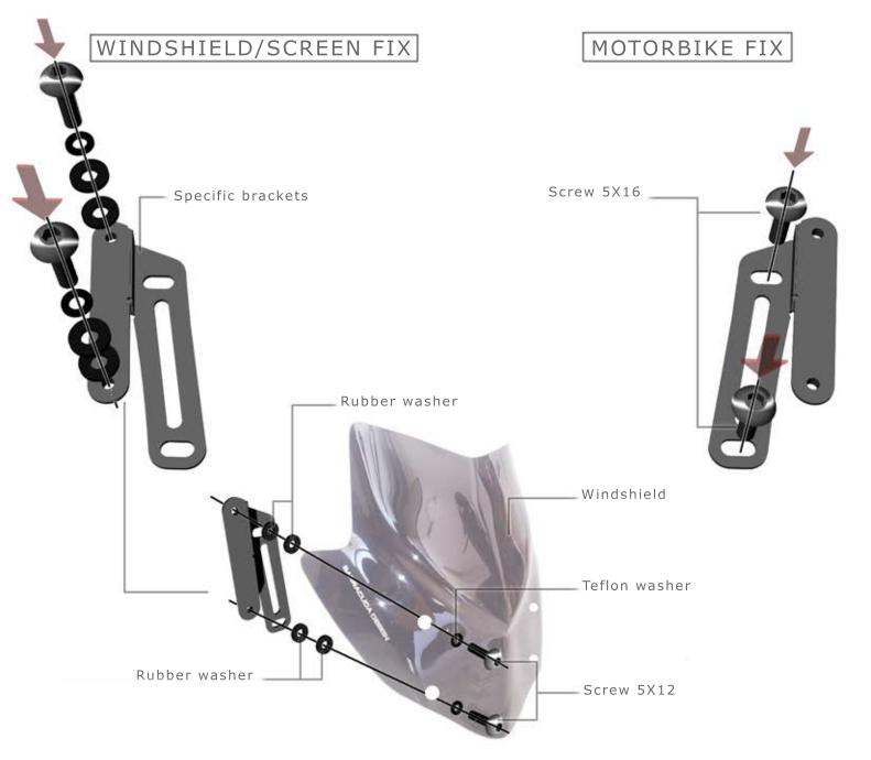
REMOVE THE ORIGINAL WINDSHIELD/SCREEN UNLOCKING THE 4 FIXING SCREWS, MOUNT THE SPE-CIFIC BRACKET WITH THE SCREWS LIKE DECRIBED UP WITHOUT LOCKING TOO MUCH THE SCREWS, MOUNT THE WINDSHIELD/SCREEN ON THE BRACKETS USING THE RUBBER WASHERS, PUT THE WINDSHIELD/SCREEN IN THE CENTER MOVING INTO ALL DIRECTIONS, REMOVE THE WINDSHIELD/SCREEN AND LOCK THE POSITION OF THE BRACKET. MOUNT THE WINDSHIELD/SCREEN. DON'T LOCK TOO MUCH TO AVOID PLEXIGLASS DAMAGES
