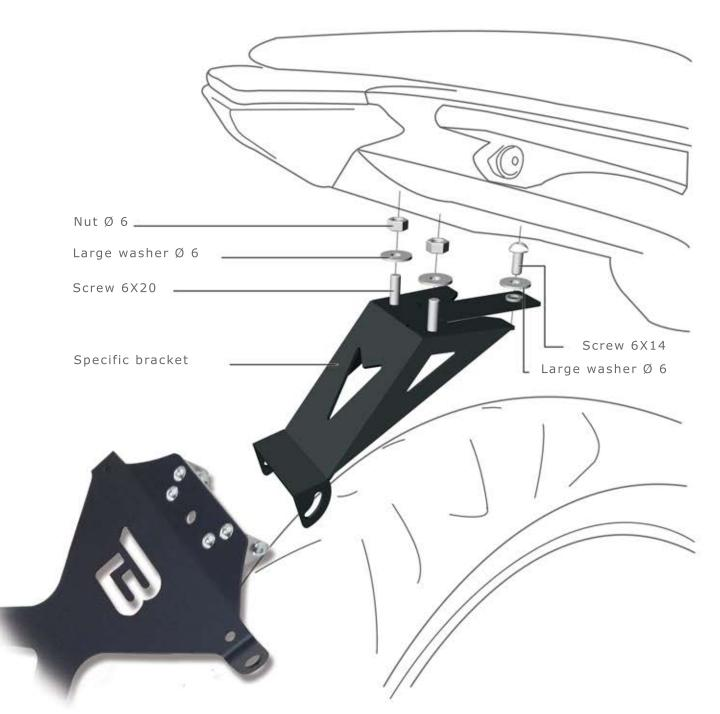
REMOVE THE ORIGINAL LICENCE PLATE. FIX THE BARRACUDA SPECIFIC BRACKET USING THE SCREWS INCLUDED LIKE SHOWN IN THE PICTURE. APPROACH AND FIX THE "X" LICENCE PLATE TO THE INSTALLED BRACKET.
