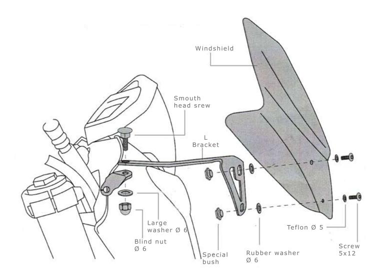
MOUNT THE WINDSHIELD/SCREEN ON "L" BRACKET LIKE DESCRIBED IN THE PICTURES. REMOVE THE FIXING SCREW FROM THE ORIGINAL STEERING PLATE AND PUT THE SHORT BRACKET USING THE ORIGI-NAL SCREWS. PUT THE WINDSHIELD/SCREEN WITH "L" BRACKET ON THE SHORT BRACKET. JOIN THE TWO BRACKET USING THE SMOUTH HEAD SCREWS, THE WASHERS AND THE BLIND NUT LIKE DESCRIBED IN THE PICTURE. POSITION THE WINDSHIELD/SCREEN AND LOCK ALL THE SCREWS.
