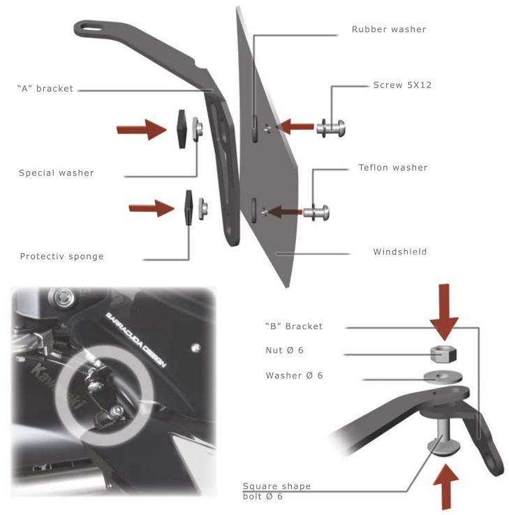
ASSEMBL THE BARRACUDA WINDSHIELD/SCREEN USING THE SCREWS AND THICKNESS INCLUDED IN THE KIT. MOUNT ALL LIKE THE INSTRUCTION, AT THE END UNLOCK THE FORK UPPER SCREWS AND SUBSTITUTE THEM WITH THE 8X50 SCREWS TOGHETER WITH THE HIGH 10 THICKNESS. WE ADVICE TO LOCK ALL TOGHETER ONCE YOU FIX THE WINDHSIELD/SCREEN TO AVOID BROKEN PART DUE TOO FORCING
