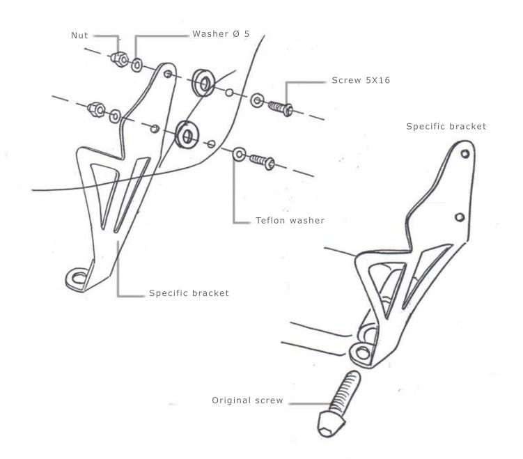
APPLY THE TWO BRACKET ON THE STEERING PLATE USING THE ORIGINAL SCREW. FIX THE WINDSHIELD/SCREEN ON THE TWO BRACKET WITH THE 5X16 SCREW LIKE DESCRIBED INTO THE PIC-TURES. FOUND THE CORRECT POSITION OF WINDHSIELD/SCREEN, LOCK ALL AND USE THE 4 RUBBER WASHER BETWEEN THE IRON BRACKET AND WINDSHIELD/SCREEN
