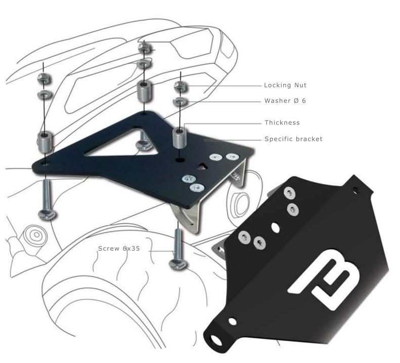
REMOVE THE ORIGINAL LICENCE PLATE FROM THE MOTORBIKE. APPLY THE BARRACUDA SPECIFIC BRACKET USING THE THICKNESS E AND SCREWS INCLUDED LIKE SHOWN IN THE PICTURE. APPROACH AND LOCK THE "X" LICENCE PLATE.
