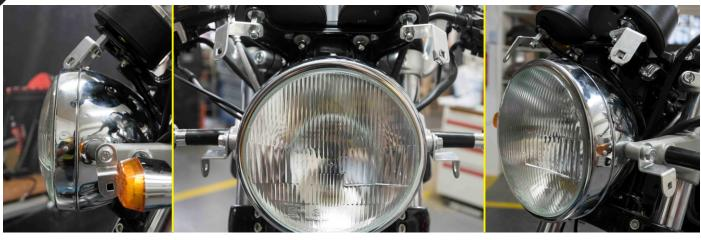
Put in place the metallic plates as you see in the above photos (4-5&6). First place the top ones on the adaptors that you have already positioned and tightened in place. Do not securely tighten them yet so that you may make any adjustments if needed. The lower metallic plates hold in place the headlight so proceed by gradually tightening them in place – try on the mask to make sure the metallic plates are in the correct position and make your adjustments before tightening.
