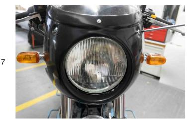
Finally place the mask in position and gradually tighten the screws in place.
