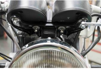
Unscrew the front end nuts that hold together the meter instruments, and in their position use the (M6X18) adaptors – as shown in the above photos 1 & 2.
