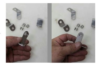
Clip the clips as shown in the left hand photo. Have a look on the next page to see how and where to place the metallic plates – we place them at the back of each metallic plate in the square hole.
