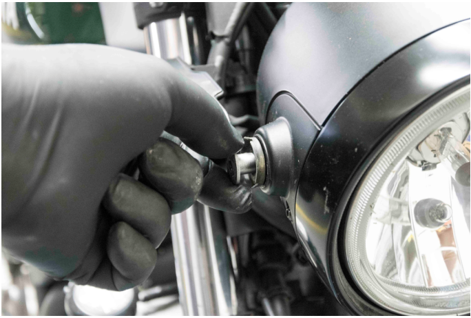
In place of the old adaptors use the new ones.
