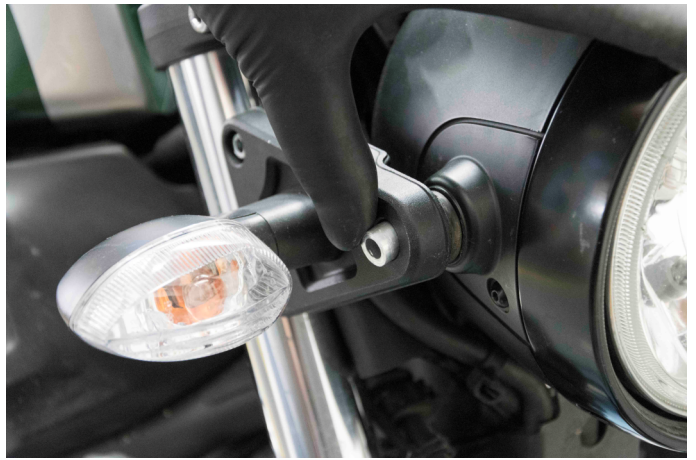
Place the headlight in position and place the adaptors on both outer sides of the headlight. You need to hold the headlight with your hands until you put the mask on.
