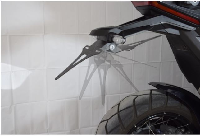
The rotation capabilities of the new License Plate Holder. You can have it in any position you want.
