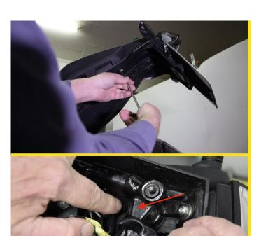
Continuing remove the four screws holding the plastic license plate extender spoiler.
