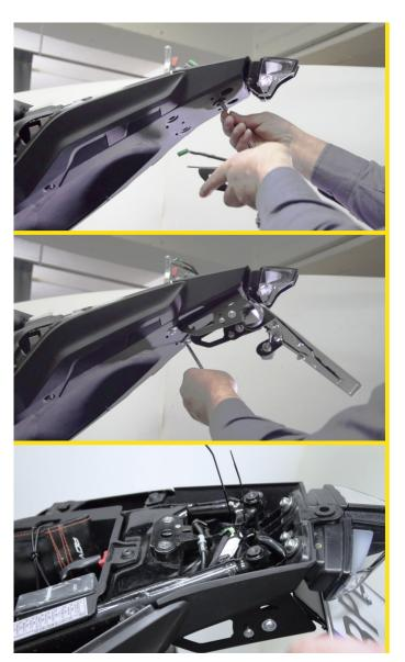
First push the flash cables through the rubber hole one by one and pull them from the above to place it in the correct position.
