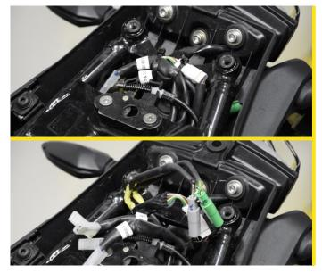
After removing the cover, you will find tied on the subframe a bundle of cables, cut the cable holders, and untangle them.
