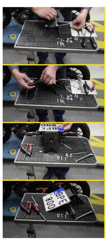
Then connect the two pieces of the new base. Follow the blueprint, on the first page to use the correct screws.
