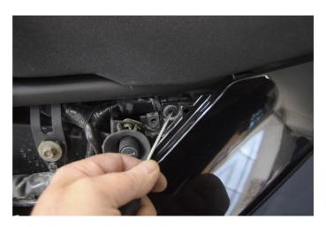
At the front, on each side it has two clips (Right and Left). Lightly press the middle pin and with a small screwdriver remove them.
