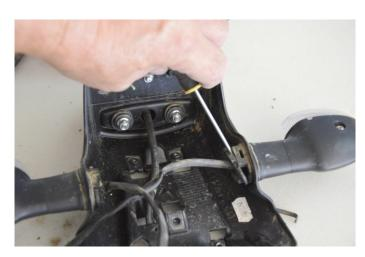
Remove the flashers above the base. Safety first and then push it through its elastic base from the hole that holds it.
