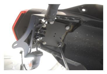
Place the base and screw it at the old possition the old base with the same screws.
