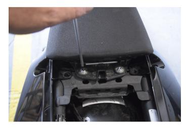
With the motorcycle key, remove the rear part of the saddle, then unscrew and remove the front part of it.
