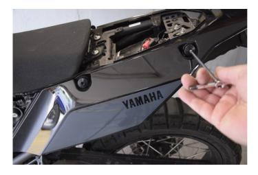
Unscrew the 4 support brackets on the sides.
