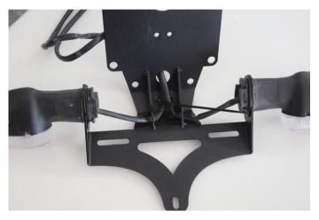
On the new license plate holder place the flashers with the same way you removed them. Remember the gray plug is for left turn signal. Make sure the cables pass through hole and put a fit to keep them tight.
