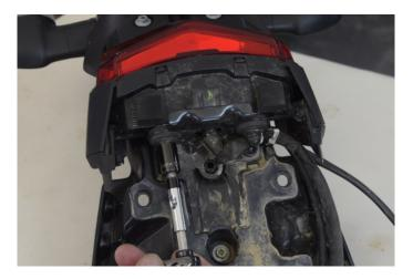
Unscrew the two screws holding the light. You will remove the rest of the base afterwards because you will use it again.
