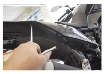
Then remove the 6 screws that are on the side/bottom part, as the photo shows.
