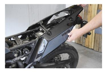
Now carefully remove the plastic cover. You will need to open it slightly at the front outwards and then backwards, because it has a clasp just above the lantern. Carefull moves are requeried so you dont break any base.
