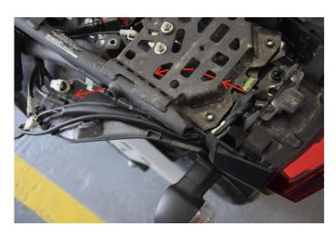
Place the wires for the flashes through the base, as the photo shows, while the cable for the light will be placed at its old position.
