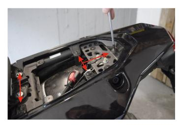
Then remove the 5 screws located on the top as shown by the arrows in the photo.
