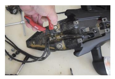
Cut the dowels that hold the wires together.
