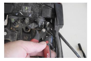
Cut the fitting that holds the taillight cable.
