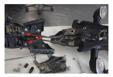
Now all the parts are separated. Also remove the base that held the lantern from the front of the base, on the screws shown by the arrows in the photo.
