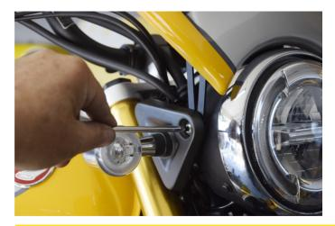
Remove the screws on the sides that hold the light.
