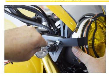
Pass the screw and mount without tightening it. Do the same on the other side.
