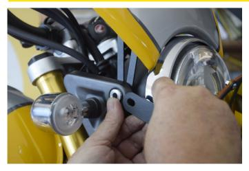
Place the large adapters on the inside side of the light base and pass the grill over it.
