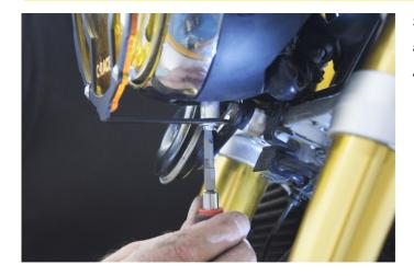
Screw the bottom screw as well, putting the small adapter between as shown in the photo. Adjust the position you want and tighten all the screws
