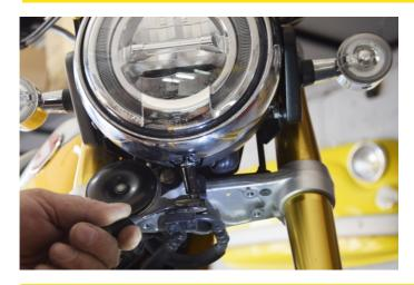
Remove the lower headlight screw adjusting the height of the light.
