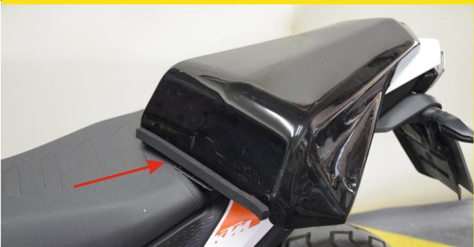
First remove the rear seat with the key.
