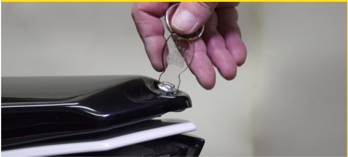
Then replace the cover and screw it in, where the rear handles were screwed.
