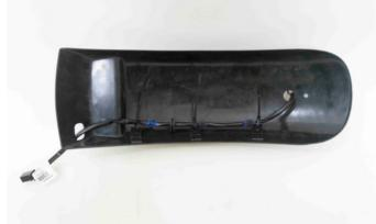
Slide the wire under the fender and hold it in place using the tireups without tightening them yet (photo 5)
