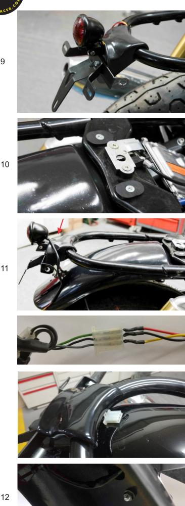
If the product you have in your hands is (RF-RE) then you will have to place the tail light as well. Place the tail light with the new base plate and the screw which protrudes from the hole that you have already drilled, align it and tighten it in place.
