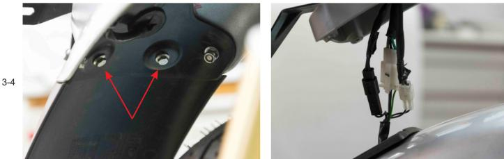
Proceed by removing the screws as shown with the arrows in photo No3. The fender will be released and all you have to do is to unclip the fuse of the tail lights
