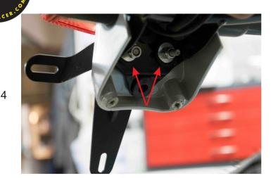
To remove the tail lights you will have to remove the 2 screws that the arrows in the left hand photo show you.
