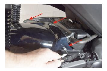
Place the new hugger where the previous one was, with the new screws as shown in the photo.
