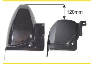
The difference of the new hugger is that it is 120mm longer than the standar and also covers the wheel on the sides, so it gives better protection.
