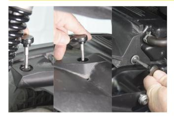
Take out the three screws that hold the rear hugger and remove it, as shown in the photo.
