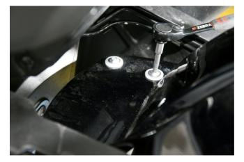
Screw the hugger to the right part as well. Before tightening all the screws make sure the fender is in the right place. If required make adjustments before tightening all screws.
