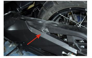
Remove the two screws indicated by the arrows, these have two mounts that hold the rear brake pipe.
