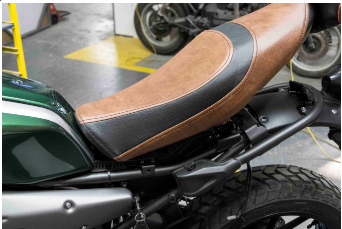
Remove the old seat using your key. And clip on the new one in the exact same way.
