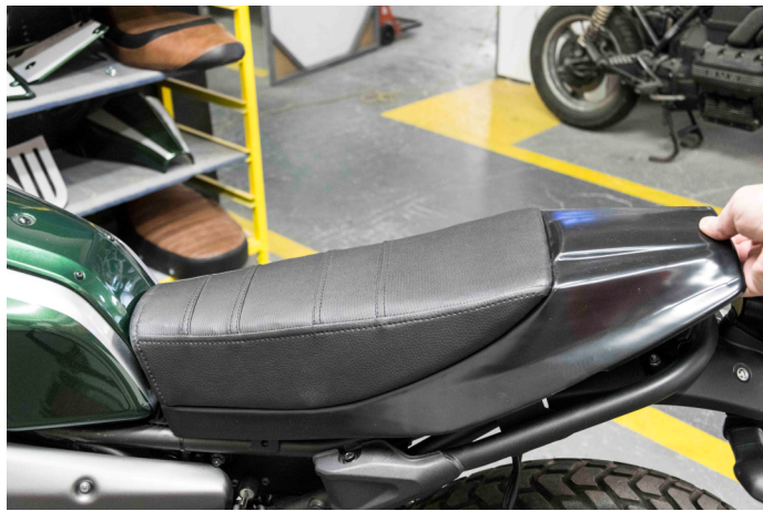
Remove the old seat using your key. And clip on the new one in the exact same way.
