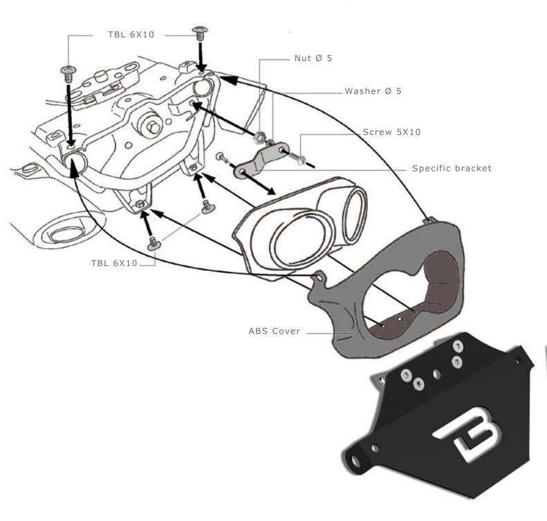
REMOVE THE ORIGINAL LICENCE PLATE FROM THE MOTORBIKE. APPLY THE ABS COVER LIKE DESCRIBED IN THE PICTURE AND THAN APPROACH THE "X" LICENCE PLATE BARRACUDA
