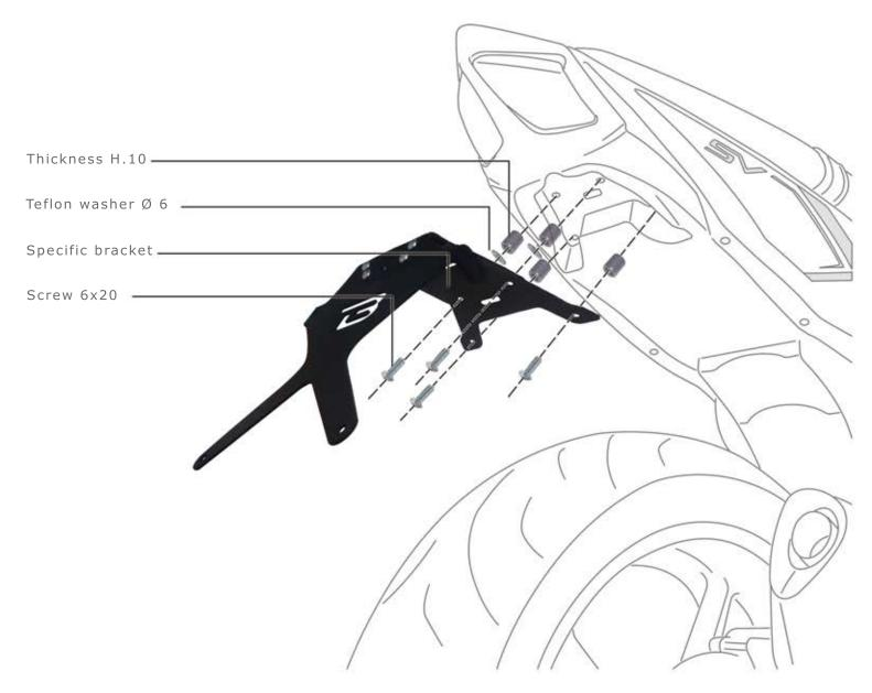
NOTE: WE ADVICE TO TAKE AN INCLINATION NOT EXCEEDING 30° TO AVOID STRUCTURAL POSSIBLE BROKEN
