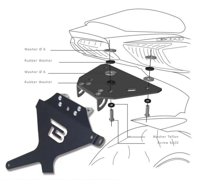
REMOVE THE ORIGINAL LICENCE PLATE FROM THE MOTORBIKE. APPLY THE BARRACUDA LICENCE PLATE FIXING IT WITH THE 6X20 SCREW INCLUDED. ATTENTION: FIX THE DIAMETER 6 LARGE WASHERS AND RUBBER WASHERS LIKE SHOWN IN THE PIC-TURE. JOIN THE LICENCE PLATE TO THE SPECIFIC BRACKET INSTALLED.
