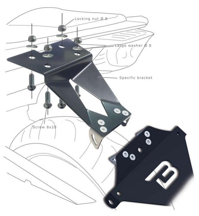
REMOVE THE ORIGINAL LICENCE PLATE AND APPLY THE BARRACUDA LICENCE PLATE IN THE SAME HOLES USING THE SCREWS INCLUDED INTO THE KIT. APPROACH AND LOCK THE "X" LICENCE PLATE BARRACUDA
