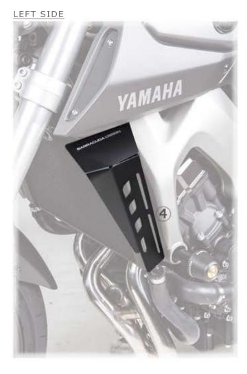
UNSCREW THE HIGHLIGHT POINTS SHOWN IN THE PICTURE (1-2-3-4) AND REMOVE THE FUEL CAP; POSITION THE BARRACUDA KIT AIR CONTROL LIKE SHOWN IN THE PICTURE;
